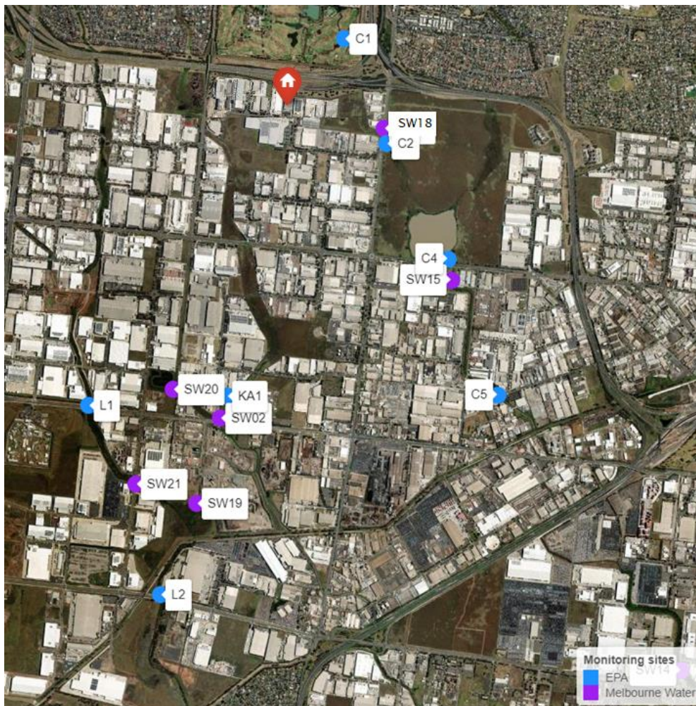
Figure 3. Location of EPA and Melbourne Water monitoring sites along the Kayes Drain, Laverton Creek and Cherry Creek waterways. Refer to Appendix A1 for list of sites and map codes. Red pin shows location of fire.
