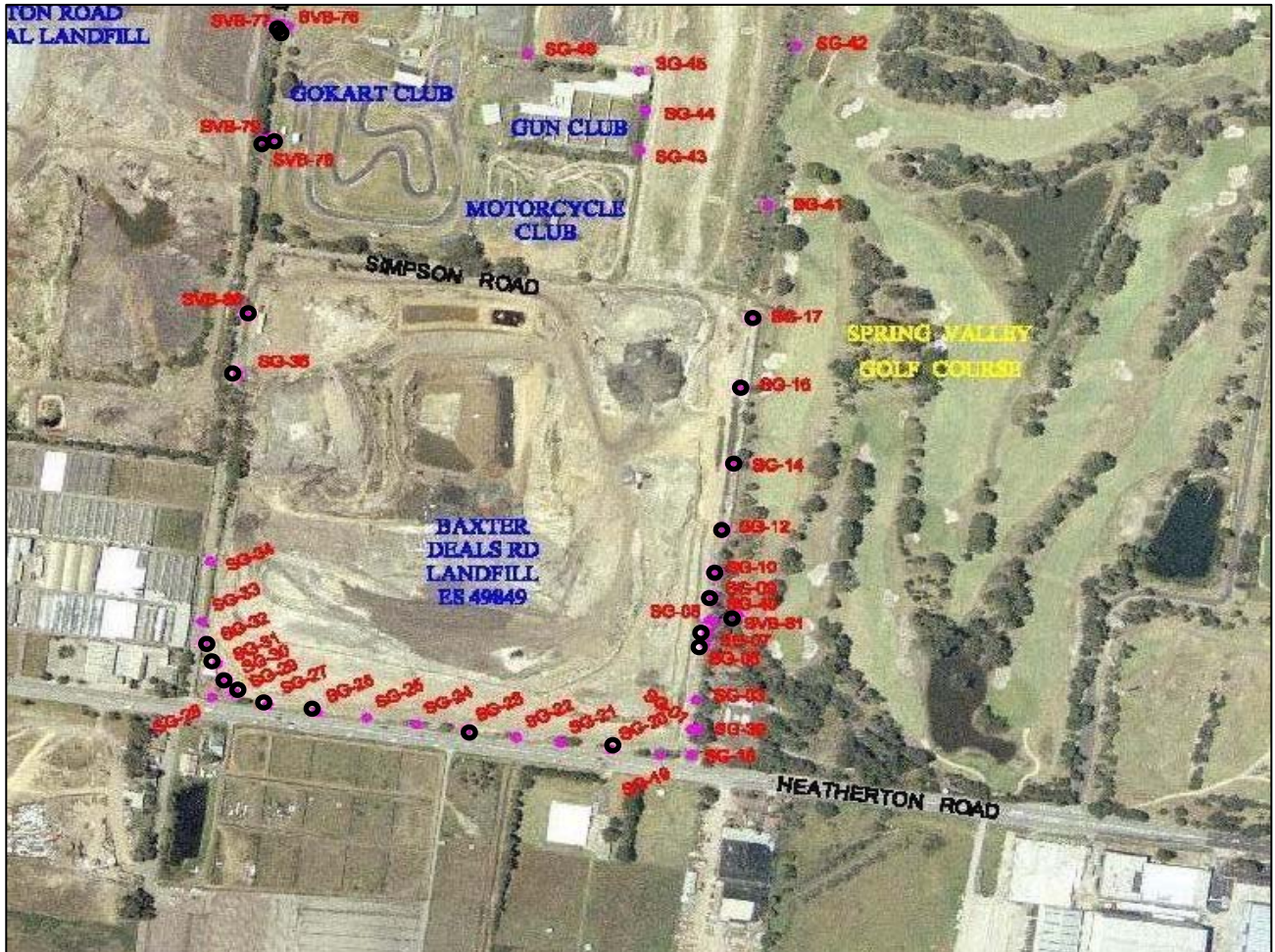
Figure: Heatherton Road probe monitoring location plan (probes used by TPI). Baxter and Cleanaway landfills shown are owned by TPI.
