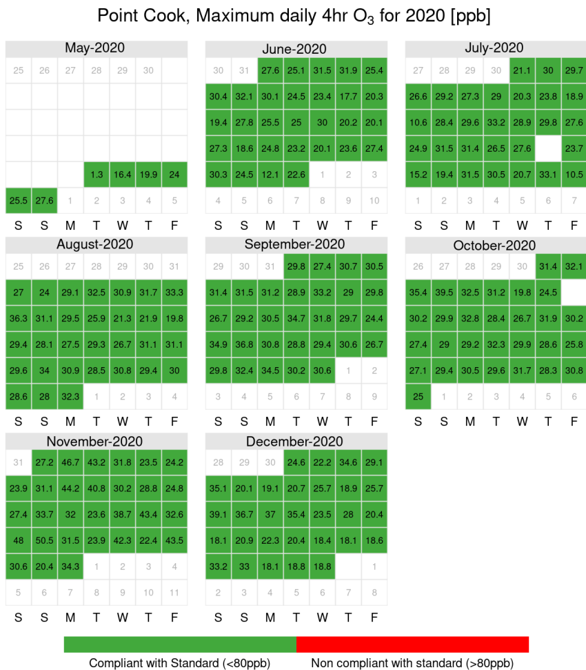
Figure 25: Point Cook 4hr O 3 calendar plots showing days where exceedances of the maximum daily standard occurred in ppb
